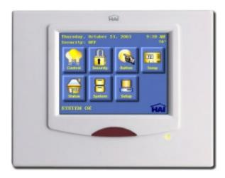
The touchscreen unit mounts flush with the wall, and is supplied with a white, beige, and almond faceplate that is a slim 3/8 inch for an elegant built-in look. OmniTouch works with OmniLT, Omni II, and OmniPro II. It connects to 4-wire console bus on the controller.
